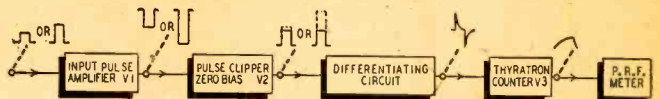
Fig. 2—Incoming wave is first amplified, then clipped and reduced to a sharp pulse.
